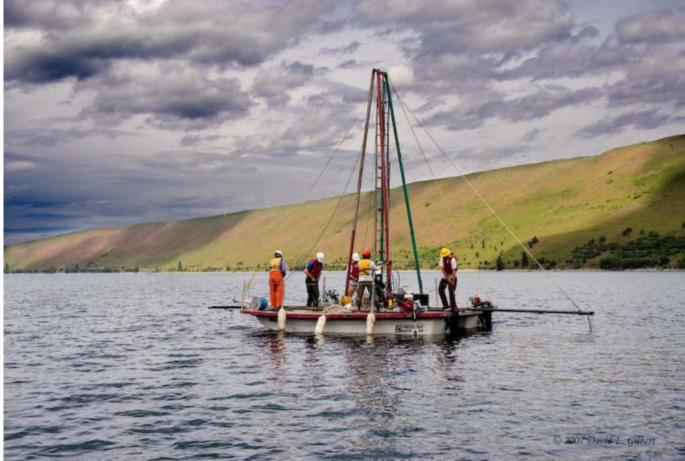
Piston coring on Wallowa Lake with a crew from the University of Alaska and the University of Minnesota. Photo by EOU president emeritus, David Gilbert.
