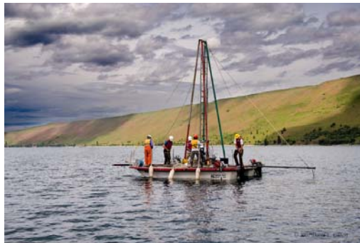
Piston coring on Wallowa Lake with a crew from the University of Alaska and the University of Minnesota. Photo by former EOU president, David Gilbert.
